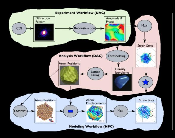
Science workflow for the comparison of a molecular dynamics simulation with a high-energy X-ray microscopy of the same material system includes three interrelated in situ and distributed area experimental workflows.
