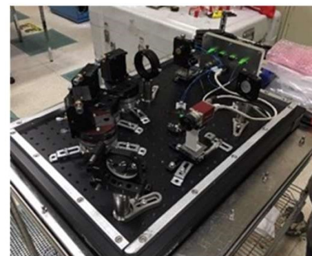
High resolution spectrometer for FM to AM mitigation
